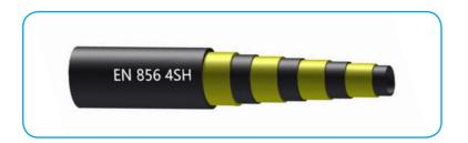
**Tube:** Inner tube in high quality synthetic rubber compounds. **Reinforcement:** Four high tensile steel wire spiraled layers.
