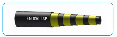
**Tube:** Inner tube in high quality synthetic rubber compounds. **Reinforcement:** Four high tensile steel wire spiraled layers.
